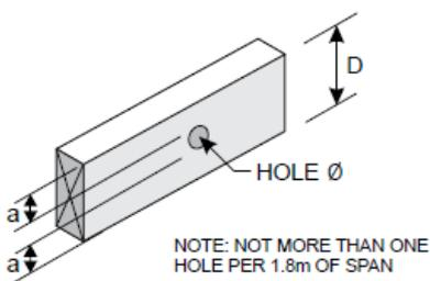
'a' min 5 Hole dia. Hole dia. max D/8
